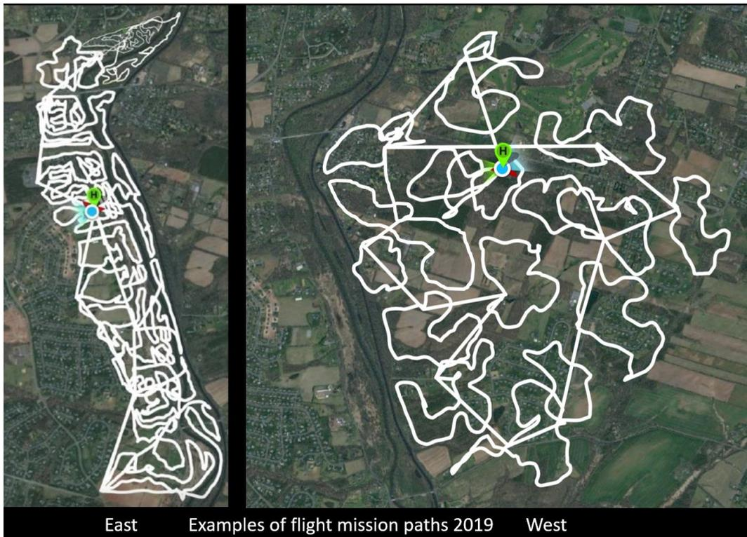
**Figure 13.** sUAS flight paths indicate sUAV flight pattern, yet also the sUAV hovers and yaws, or turns radially, to “see” in different directions.
