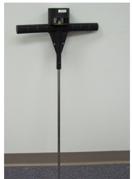
A hand-held penetrometer. The device is about 37 inches tall and has a dial on the top which reports soil strength in pounds per square inch.
